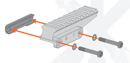
Secure screws using a T25 bit driver. Lightly snug all screws before applying final torque to any. DO NOT EXCEED 35 IN-LBS.
